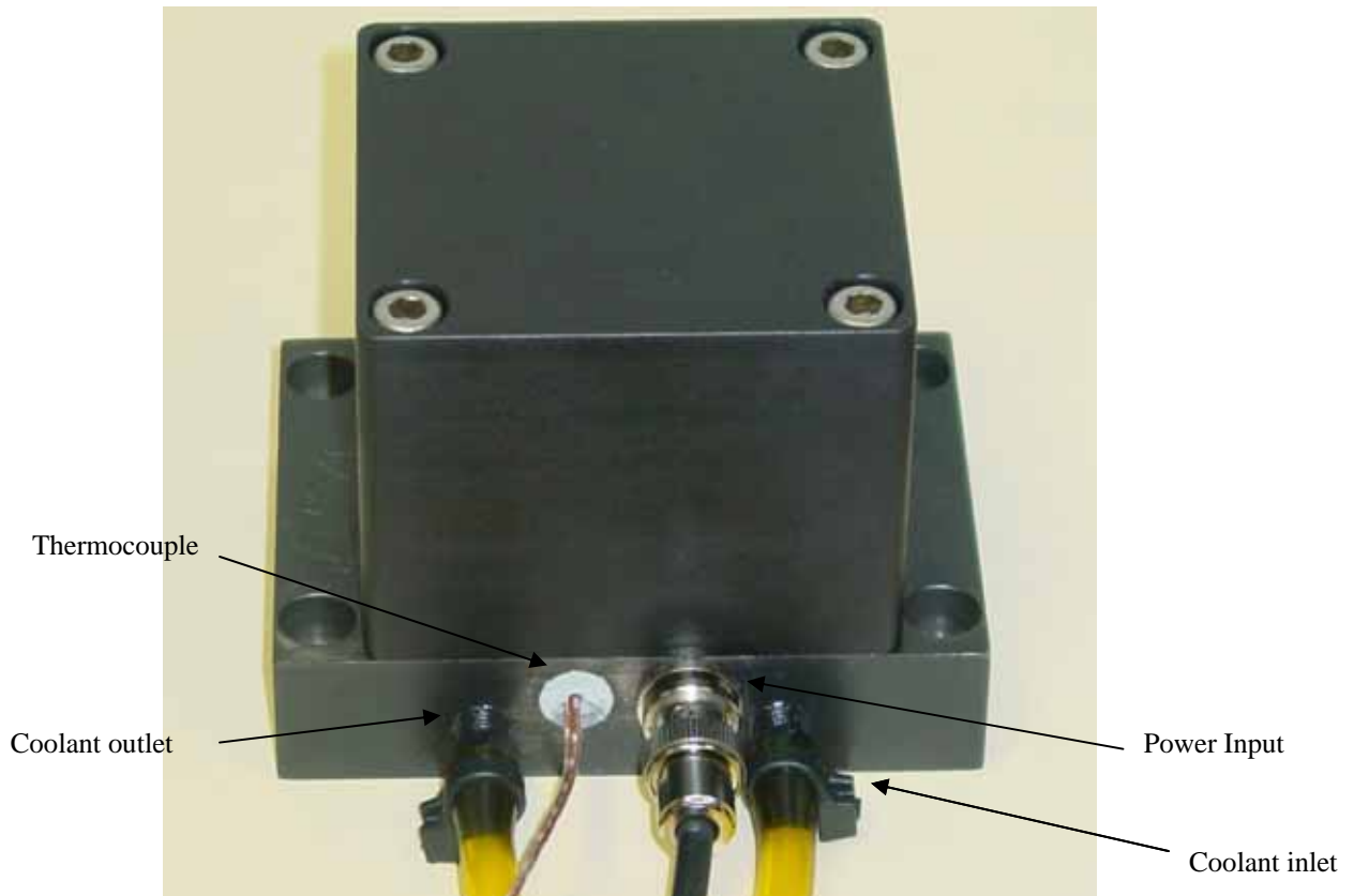
RFTS "HEAD" Rear View
