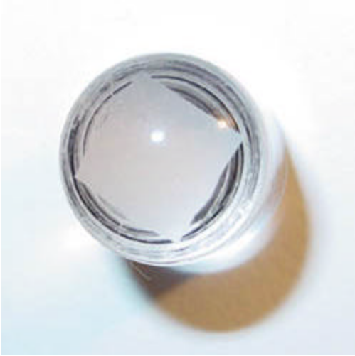
Square Profile Cut While Spindle Rotates at High Speed
